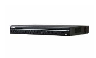
Dahua's new 5000 series network video recorder delivers excellent performance and high recording quality that is ideally suitable for IP video surveillance applications. This professional NVR adopts powerful processor, providing the capability of 4K resolution processing for applications where image details are highly required. Additionally, the NVR can be served as edge storage, central storage or backup storage with an intuitive shortcut operation menu for remote management and control
